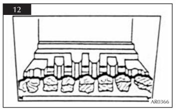
6.10 Place three large coals on the front coal so that they lean against the flame baffle, and the four large coals on the flame baffle so that they sit on the fingers, see diagram 13.
